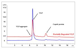
**Resin:** Monomix MC10 SEC-500 (10 μm, 500 Å) **Column:** 7.8 x 300 mm (Stainless Steel)
