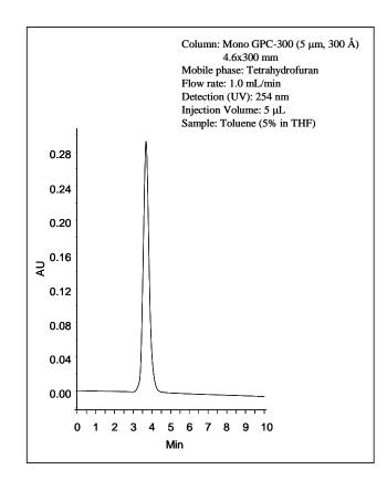
Figure 1. Toluene is used to test the column for quality control.
