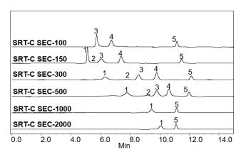
Figure 1. Elution profiles of a protein mixture by SRT-C SEC-100, SRT-C SEC-150, SRT-C SEC-300, SRT-C SEC-500, SRT-C SEC-1000, and SRT-C SEC-2000 columns:  $5\mu$ m, 7.8x300mm; Mobile phase: 150 mM Sodium Phosphate buffer, pH 7.0; Flow rate: 1.0 mL/min; Detection: UV 214 nm; Temperature: ambient (23 °C); Injection volume:  $5 \mu$ L.
