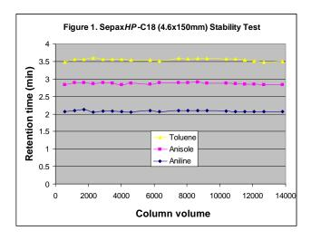
Such high stability allows SepaxHP-C18 extremely suitable for validation of various analytes. The unique mono-functional bonding chemistry for SepaxHP-C18 avoids the formation of multiple C18 layers. Such uniform stationary phase allows the separation to achieve high selectivity and high efficiency. A typical test chromatogram for quality control is shown in Figure 2 for a 4.6x150mm SepaxHP-C18 column.
