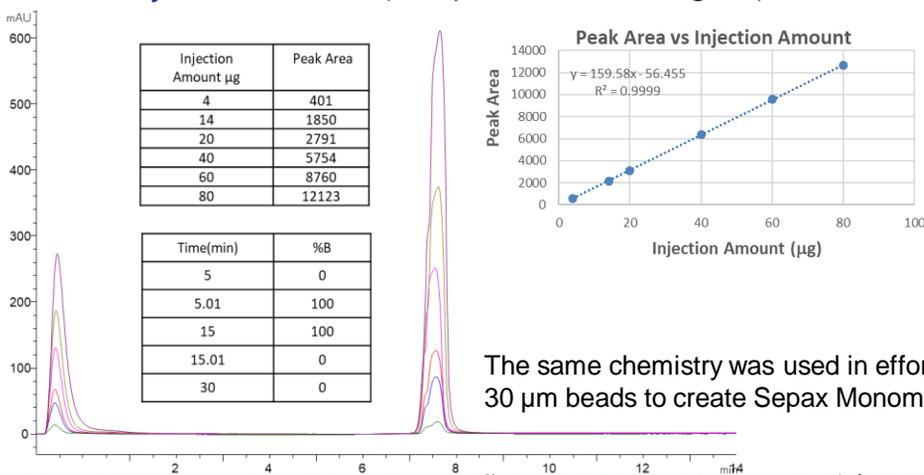
Column: HPLC Column packed with Sepax Monomix Affinity HSA Bulk Media 2.1 x 50 mm PEEK (P/N: 272201P-2105); Mobile phase A: 20mM phosphate,150mM NaCl, pH 7.5; B: 0.1 M Glycine, pH 2.5; Flow rate: 0.4 mL/min. 0-5 min 100%A, 5.1 to 15 min 100%B, 15.1 to 35 min 100%A; Detector: 280 nm; Column temperature: 25 ° C
