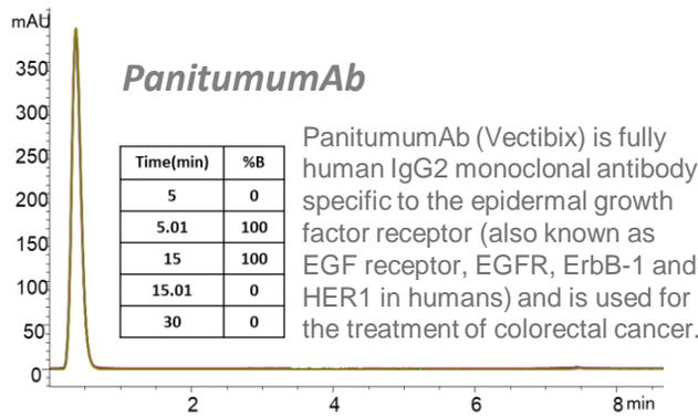
Column : Sepax BioService Affinity HSA 2.1 x 50 mm PEEK (P/N: 272101P-2105); Mobile phase A: 20mM phosphate,150mM NaCl, pH 7.5; B: 0.1 M Glycine, pH 2.5; Flow rate: 0.5 mL/min; Detector: 280 nm; Column temperature: 25 ° C; Sample: 2 mg/mL; Injection Amount: 10 µL
