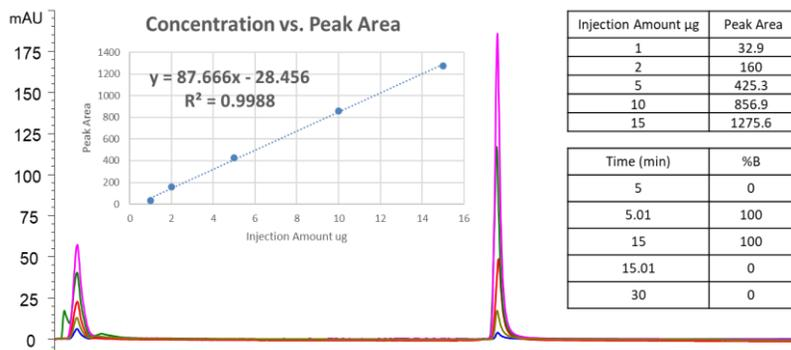
Column : Sepax BioService Affinity HSA 2.1 x 50 mm PEEK (P/N: 272101P-2105); Mobile phase A: 20mM phosphate,150mM NaCl, pH 7.5; B: 0.1 M Glycine, pH 2.5; Flow rate: 0.5 mL/min; Detector: 280 nm; Column temperature: 25 ° C
