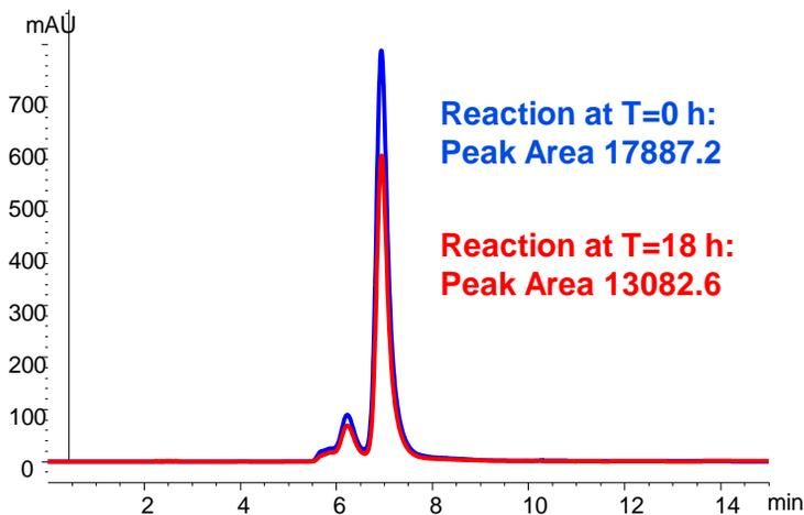
Column to Monitor Reaction: HPLC Column, Sepax, Zenix SEC-150, 3µm, 150 A 4.6 x 300 mm (P/N: [213150-4630](#)); Mobile phase: 150 mM sodium phosphate, pH 7.0; Isocratic: 15 min; Flow rate: 0.35 mL/min; Detector: 280 nm; Column temperature: 25 °C; Injection 5 µL
